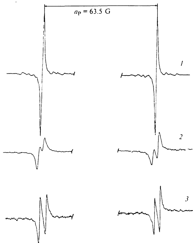
Fig. 6. ESR spectra of the \text{C}_{60}\text{P}(\text{O})(\text{OPri})_2 radical at various temperatures (K): 300 (1), 233 (2), and 200 (3).
